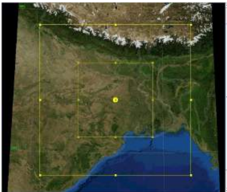
Figure 5.4: AERMOD grid covering the Jharia Coal Fields (JCF). The line, area, and point sources covered in the study are indicated in red color. The UTM coordinates of the left bottom point are x=406111 and y=2603492 , and the coordinates of the right top point are x=456248 and y=2653417 .
