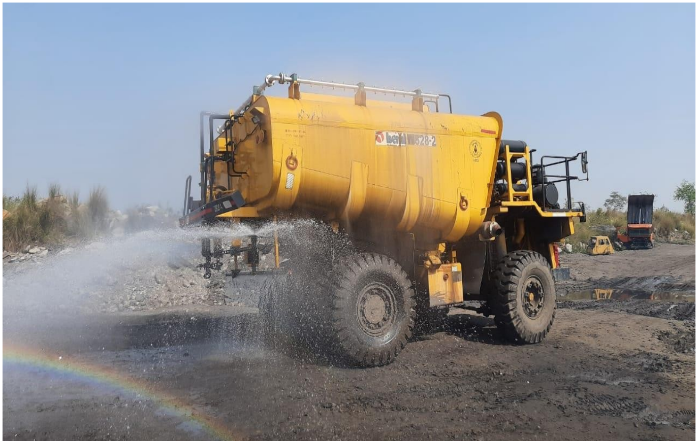
Water Sprinkling on Haul roads within mines through Mist type water tanker (28 KL Capacity)
