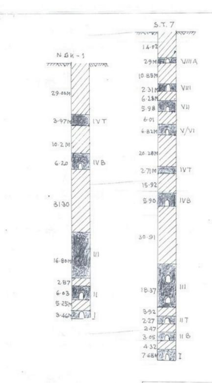
B.C.C.LTD. LODNA AREA B.H.SEC.OF PROPOSED HIRED PATCH'A' OF NT-ST O.C.P. NOT TO SCALE
